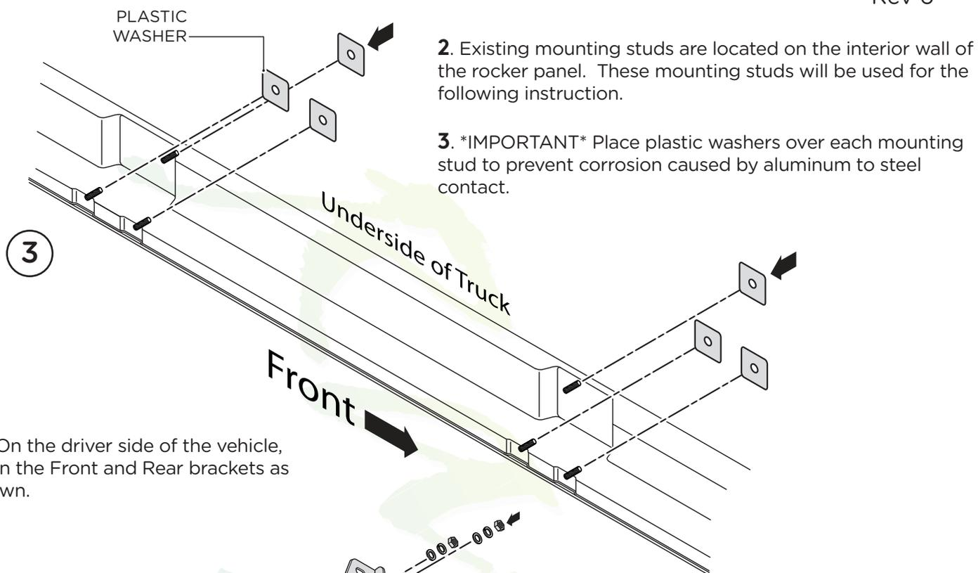
4. On the driver side of the vehicle, align the Front and Rear brackets as shown.
